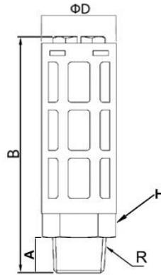
Body (noise absorbing material): Polyethylene
