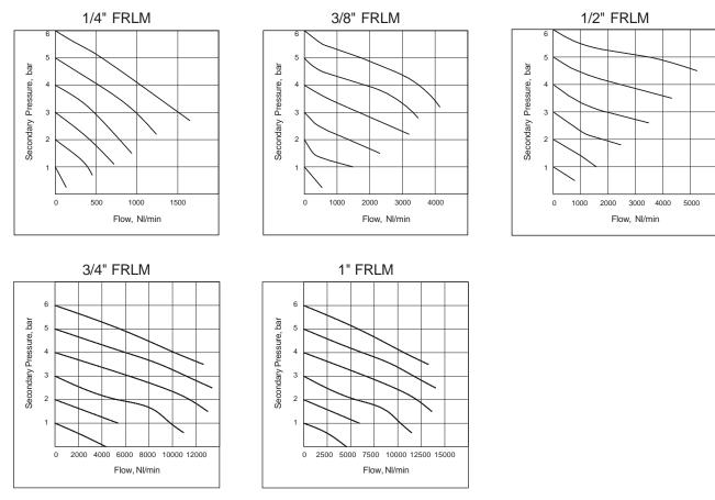
Flow graphs are for 40µm filterations only
