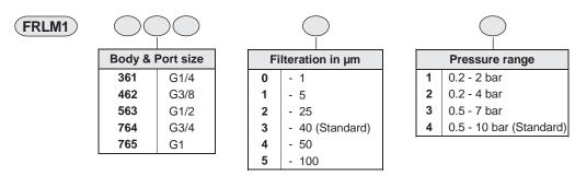
Ordering example : Filter Regulator Lubricator Modular - 3/8 (with G3/8 port size ) with 5µm Filter and pressure range 0.5 - 7 bar: Ordering No: FRLM 146213.
