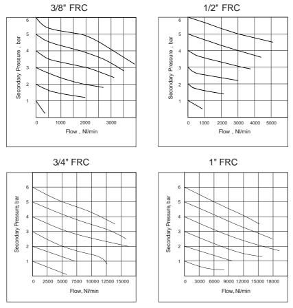
Flow graphs are for 40µm filterations only
