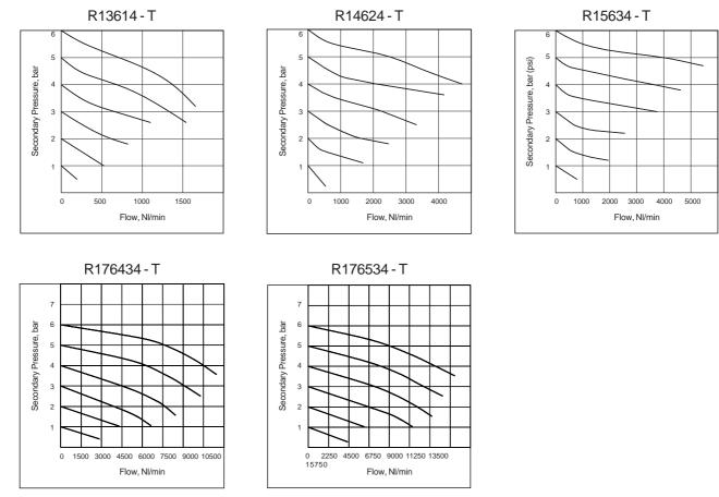
Flow graphs are for 40µm filterations and 10 bar pressure.
