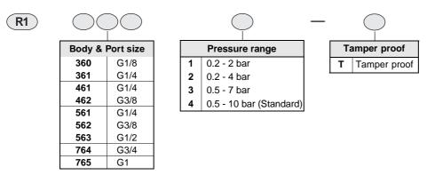
Ordering Example :- Regulator - 3/8 size ( with G3/8 port ), with pressure range 0.5 - 7 bar with Tamper proof : Ordering No : R14623-T. If ordered as 3/8 Regulator, our standard model R14624, G3/8 with pressure range 0.5 -10 bar will be supplied.
