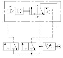
Z - Pulse input "count"Y - Pulse input "reset"
